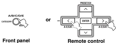
To change the preset number (1 to 8), press PRESET/TUNING/CH </> (or PRESET/CH ^ / v on the remote control) repeatedly.
