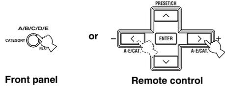
To search a channel within the selected channel category, press **PRESET/TUNING/CH** </> (or **PRESET/CH** ^ / ∨ on the remote control) repeatedly.
