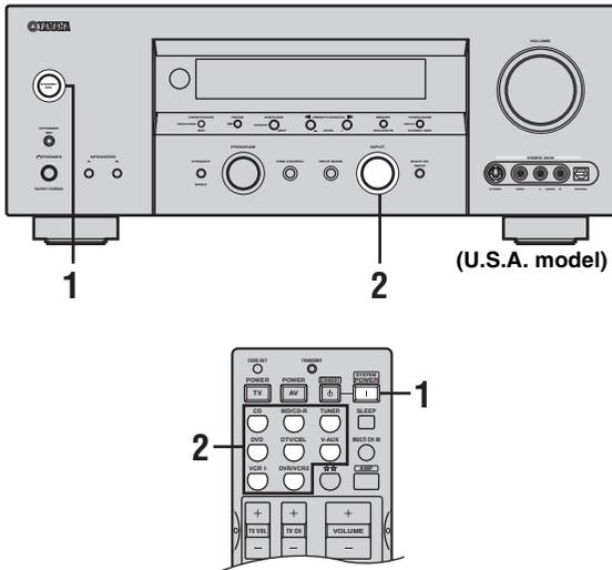
**1 Turn on the power of this unit and all connected components.**
