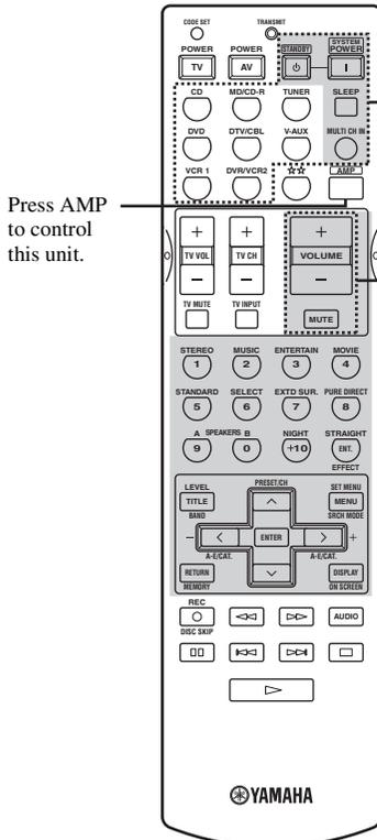
The buttons in the dotted lines control this unit in any mode (SYSTEM POWER, STANDBY, SLEEP, MULTI CH IN, VOLUME +/-, MUTE and input selector buttons) function in any mode.
