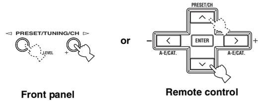
You can search a channel with the quick search by pressing and holding **PRESET/TUNING/CH** </> (or **PRESET/CH** ^ / ∨ on the remote control).
