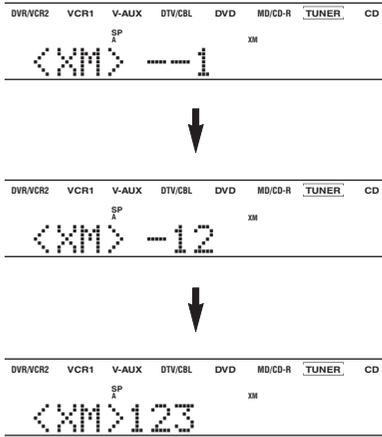
**4 If you enter fewer than three numbers, you may press ENT. to tune to the channel immediately or wait a few seconds to confirm the entered channel number.**
